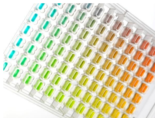
A 4 corner gradient plate for protein crystal optimisation created using TTP Labtech's dragonfly.
