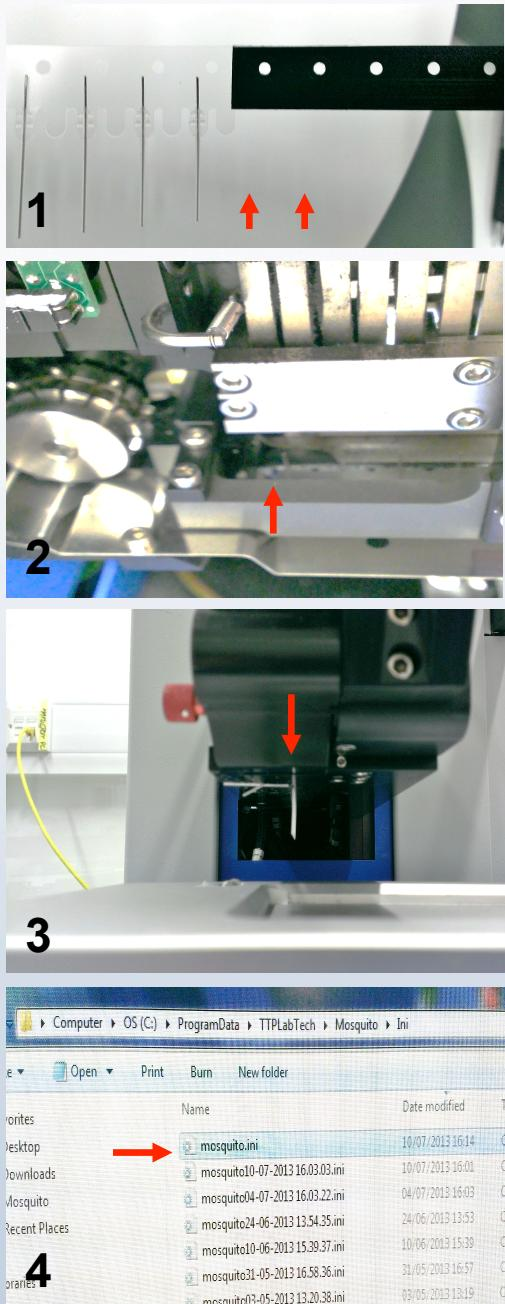
**Reloading a spool.** When things go wrong (especially the phase), the best thing to do is probably to proceed with reloading the spool. For that you need to place a spare black-leader-tape on the spool: make sure you cut the side of the tape along with the first couple of tips (Figure 1).
