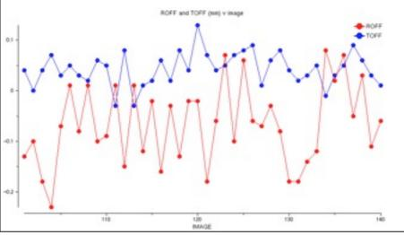
Results in instability in refinement of detector parameters.
