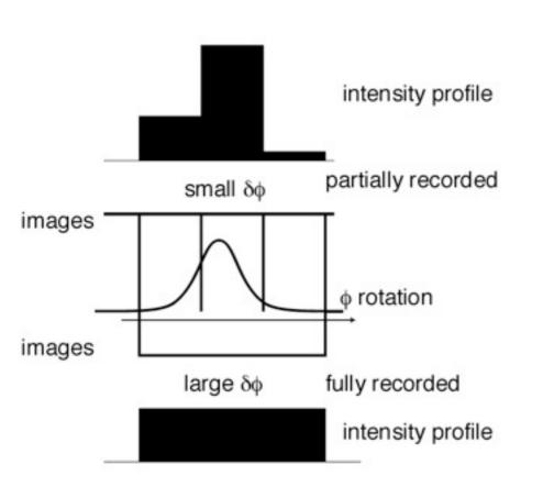
Depending on the slice width and the reflection width a reflection may occur on one image (full or fully recorded) or on several (partial or partially recorded)
