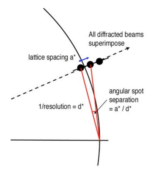
When a closely-spaced row of spots (eg along  $a^*$ ) is moving perpendicularly into the sphere, their diffracted beams almost coincide. The spots are on top of each other on the detector, and are only separated on  $\phi$
