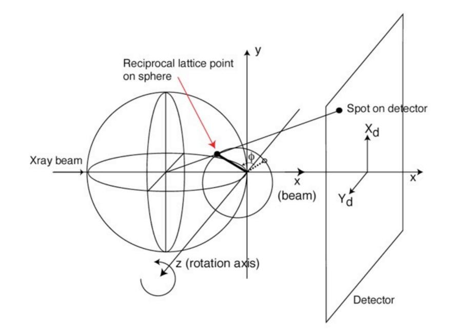
As the crystal rotates, each lattice point in turn passes through the sphere, and a spot is recorded on the detector We can use the Ewald construction to understand
