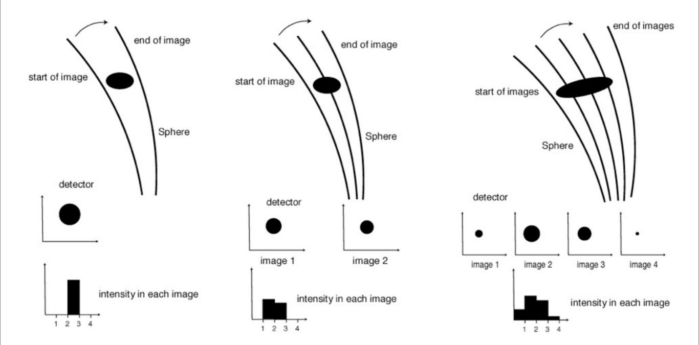
A fully-recorded spot is entirely recorded on one image Partials are recorded on two or more images "Fine-sliced" data has spots sampled in 3-dimensions
