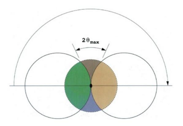
To use the Ewald sphere construction to understand which parts of reciprocal space are measured, it is easier to fix the "resolution sphere" of all reciprocal lattice points within a maximum resolution, and to rotate the Ewald sphere. The region collected is the volume swept out by the leading and trailing surfaces of the sphere
