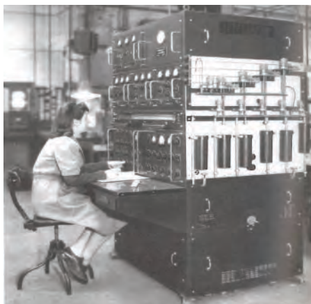
Metropolitan Vickers MS1 Mass Spectrometer 1946
