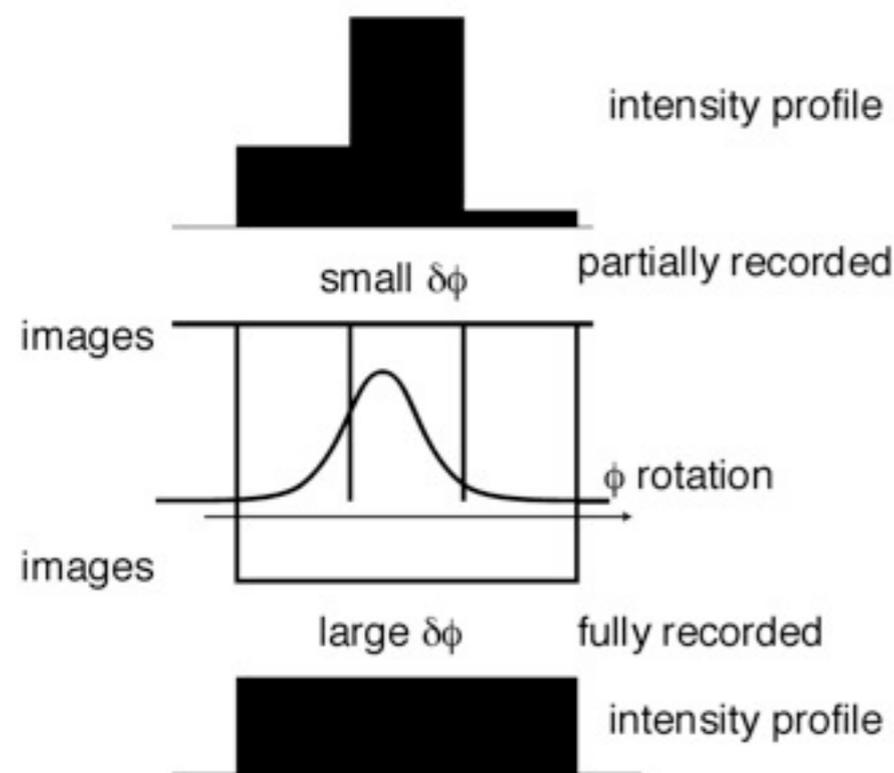
Depending on the slice width and the reflection width a reflection may occur on one image (*full or fully recorded*) or on several (*partial or partially recorded*)
