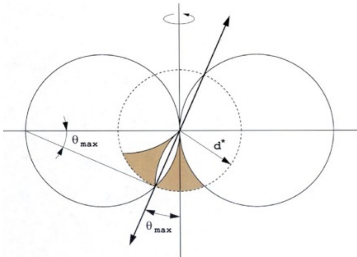
The blind region may be filled in by collecting a second set of data, offsetting the crystal by at least  $\theta_{\max}$  or by symmetry (except in PI)
