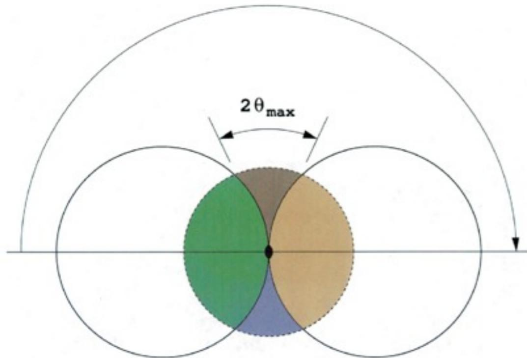
To use the Ewald sphere construction to understand which parts of reciprocal space are measured, it is easier to fix the “resolution sphere” of all reciprocal lattice points within a maximum resolution, and to rotate the Ewald sphere. The region collected is the volume swept out by the leading and trailing surfaces of the sphere
