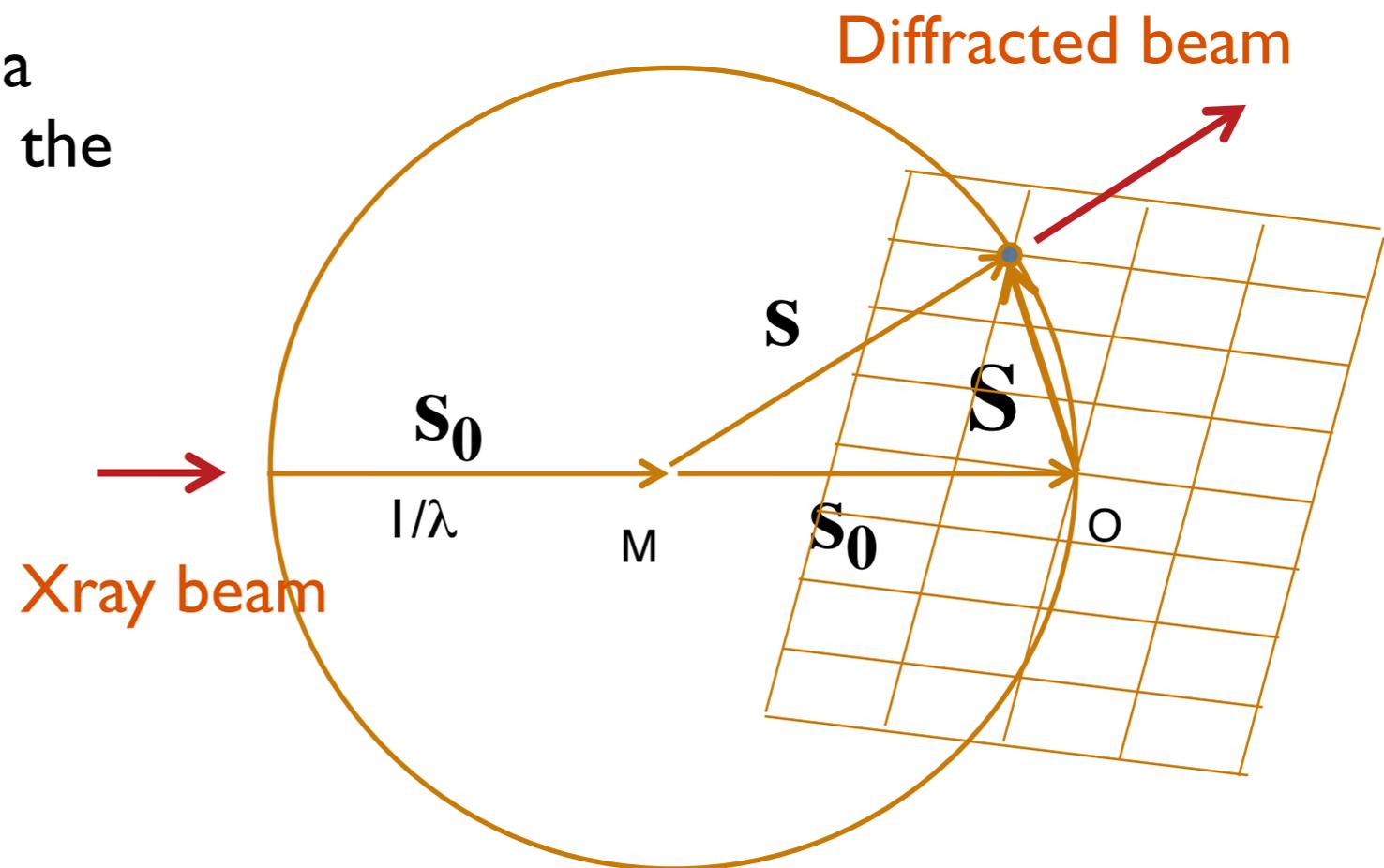
As the crystal rotates, so does the the reciprocal lattice
