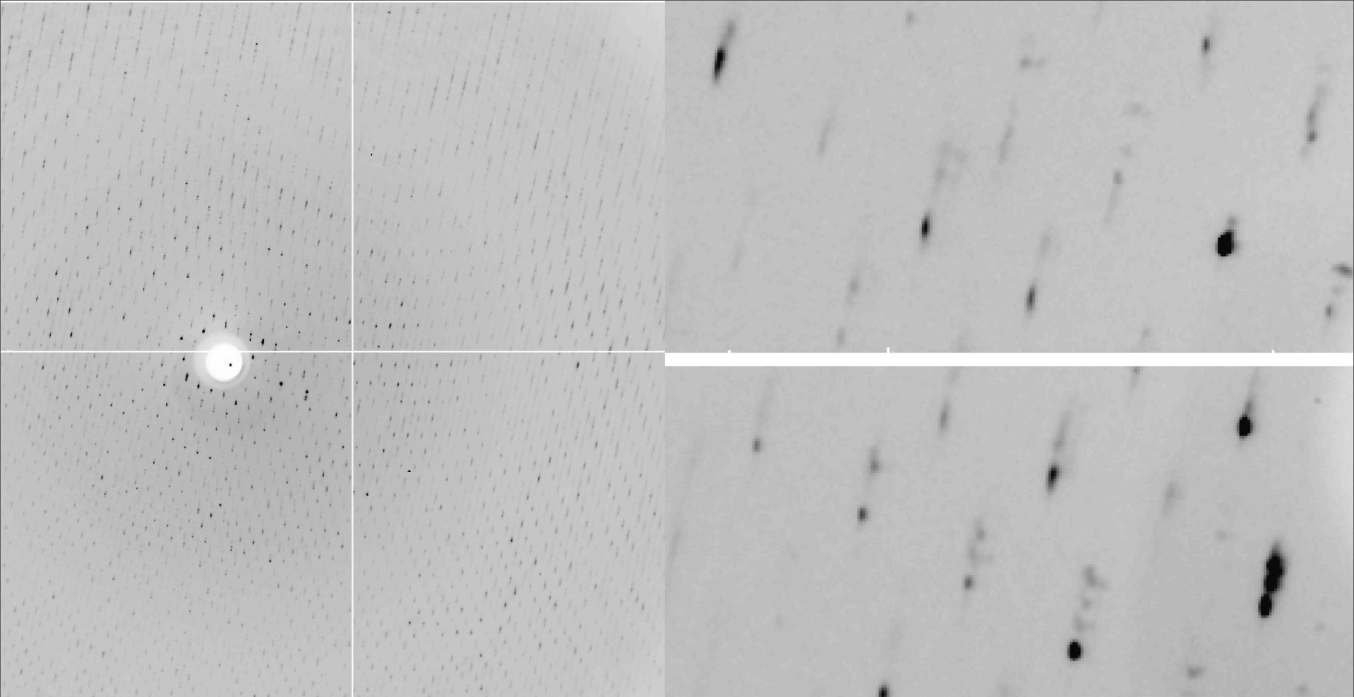
Spots not resolved, very poor spot shape and streaking
