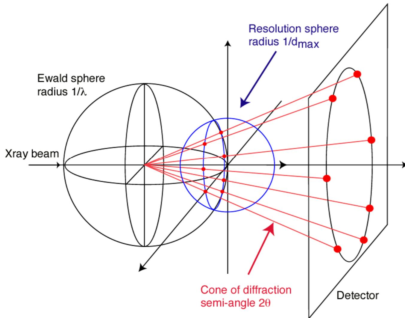
For a maximum resolution of  $d_{\max}$ , all diffraction vectors  $\mathbf{S}$  must lie within a resolution sphere of radius  $1/d_{\max}$
