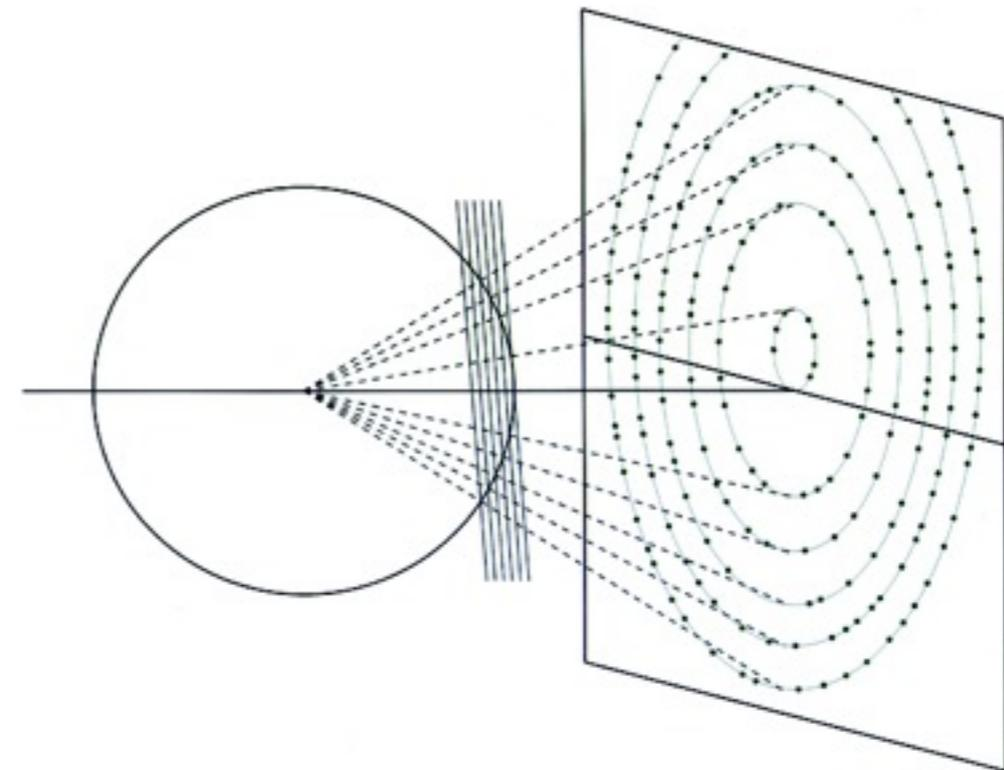
If the crystal is rotated through a small angle, each circle is broadened into a *lune*. All the spots in a lune belong to one plane of the reciprocal lattice (not necessarily a principal plane)
