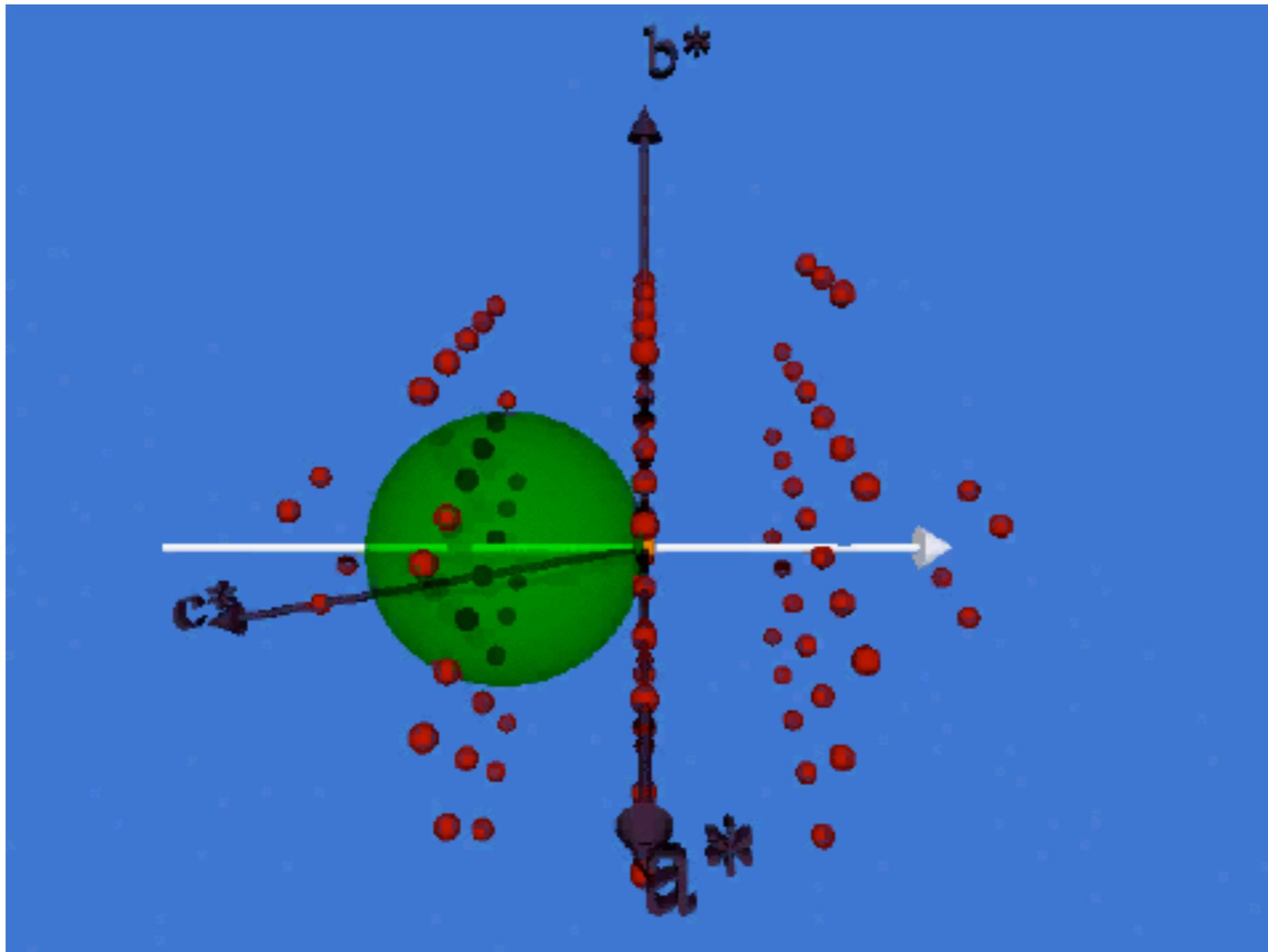
The part of the reciprocal lattice which intersects the sphere is projected on to the detector
