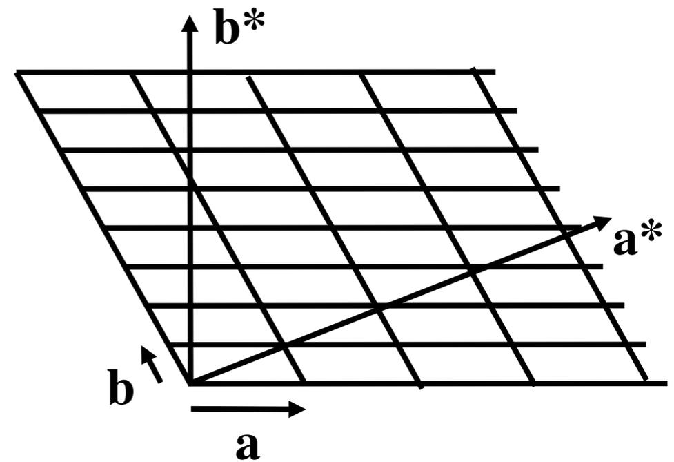
The reciprocal lattice vectors are perpendicular to the *planes* of the real crystal lattice, since the scattering can be considered as coming from reflecting planes (the Bragg planes)
