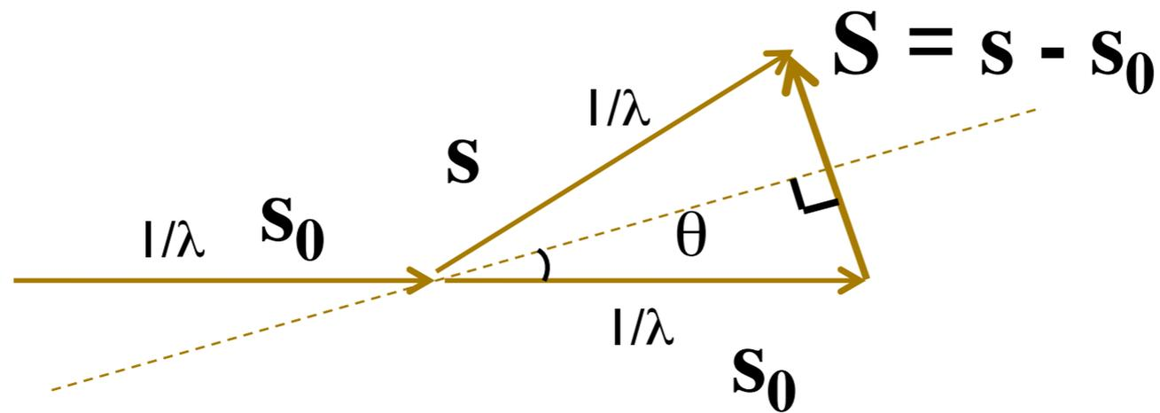
The general condition for diffraction is illustrated by the vector equation
