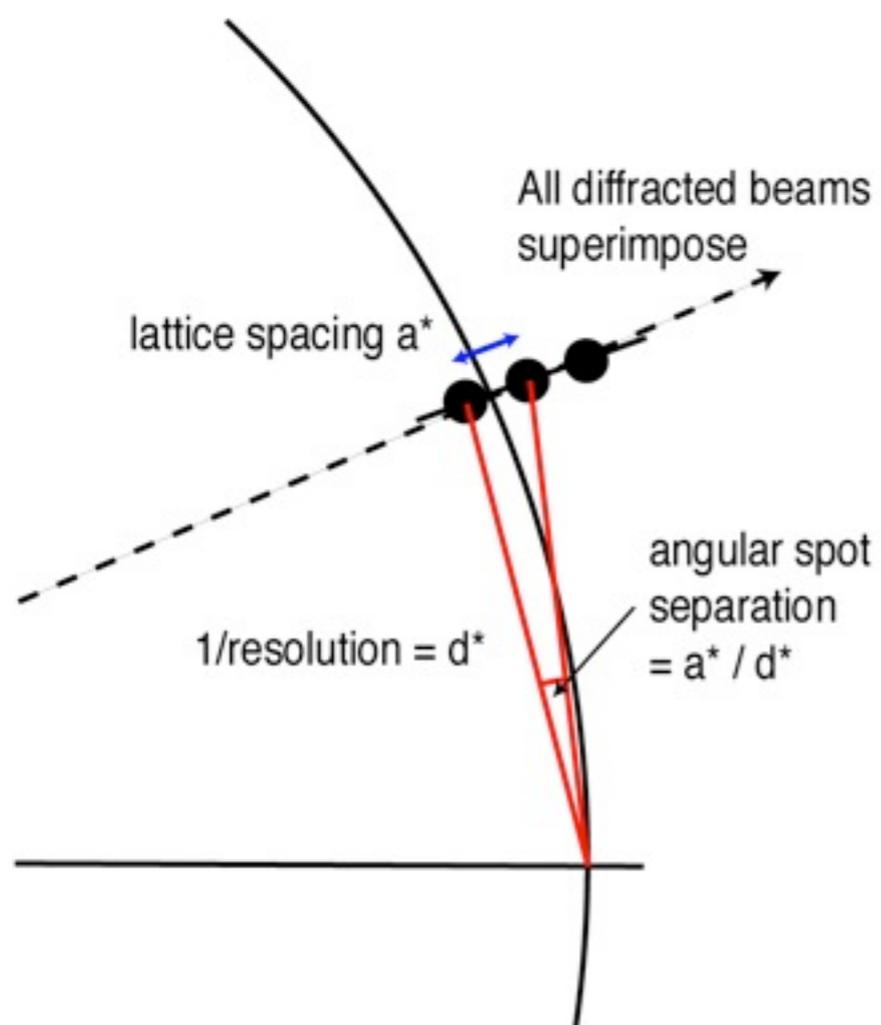
When a closely-spaced row of spots (eg along  $a^*$ ) is moving perpendicularly into the sphere, their diffracted beams almost coincide. The spots are on top of each other on the detector, and are only separated on  $\phi$
