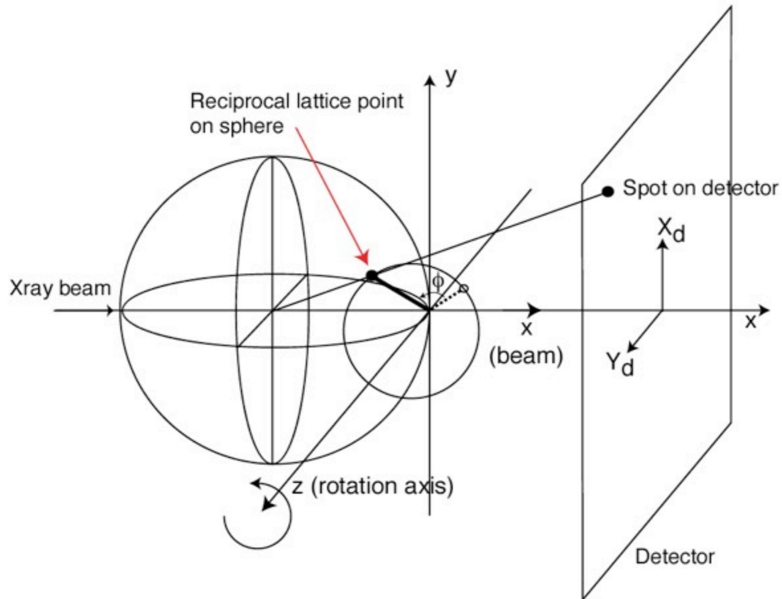
As the crystal rotates, each lattice point in turn passes through the sphere, and a spot is recorded on the detector
