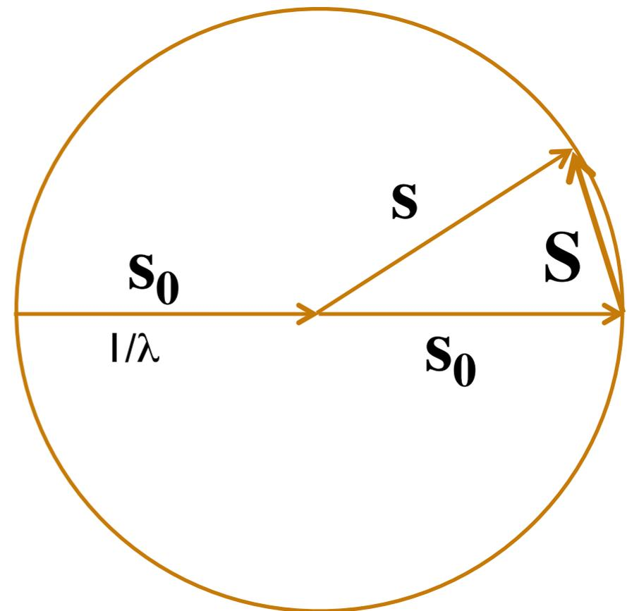
The Ewald sphere is only a construction but is very useful to understand the *geometry* of diffraction. Confusingly, it has two origins:-
