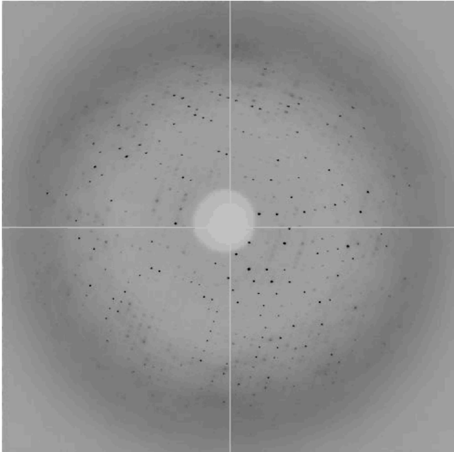
The full diffraction pattern (ie the reciprocal lattice) is 3-dimensional, and we want to measure the whole sphere to the maximum resolution (radius) available.
