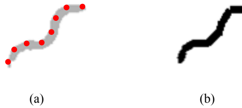
Figure 5.8: (a) 8 joint points chosen manually for the 7 parts in this frame, (b) body pose built from manually selected joint points.
