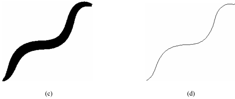
Figure 1.4: (a) Gray level image acquired from a video sequence. (b) Corresponding binary image after thresholding. (c) Binary image after hole filling and closing operator. (d) Skeleton after skeletonizing and pruning algorithm.
